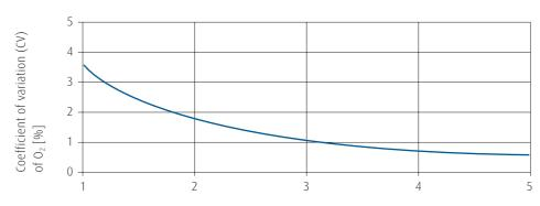
Distance from oxygen injection, based on air pipe diameter D
