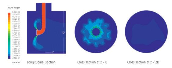
Example of CFD simulation of an OXYMIX™ Oxygen distribution in longitudinal and cross sections Operating data: air velocity 5 m/s, oxygen enrichment 24 vol.-%
