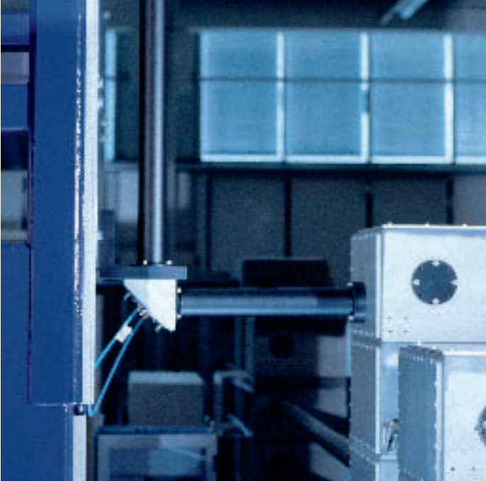
Fig. 16: Beam guidance system with a processing head
