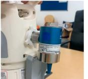
Once the regulator has been plugged into the cylinder, attach your tubing to outlet valve on the regulator, not the outlet valve on the cylinder (as shown in the picture below). Then turn the cylinder hand wheel anticlockwise, until it comes to a complete stop.
