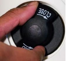
1. Turn off the cylinder by rotating the hand wheel to zero. clockwise until it comes to a stop.
