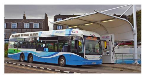
The site has the capacity to produce 360kg of hydrogen daily. That is enough for the current fleet of 10 x 42-seat buses to travel up to 350km each day emitting nothing more than clean water produced from the tail pipes.
