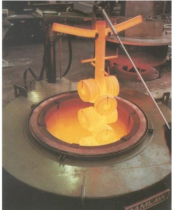
Figure 2. Parts being withdrawn from a pit furnace for quenching
