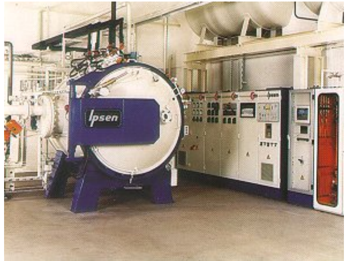
Figure 5. A vacuum furnace used for hardening tools
