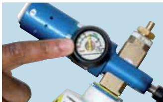
**4.2** Check the contents gauge at regular intervals to ensure there is sufficient gas for continued use.
