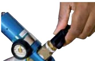
**3.10** Check for leaks by listening for a hissing sound. If you suspect a leak, shut off the valve.
