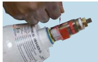
**2.3** Remove the tamper evident seal by pulling the tear strip. Discard the seal and remove the plastic clip. **The seal and clip will not be present if the cylinder has been used before.**
