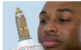
**2.4** Inspect the valve to ensure it is undamaged, free from oil and grease and clean. **If the valve appears contaminated or damaged it must not be used. Contact BOC to arrange for its return and replacement.**
