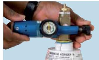
**3.4** Engage the pins on the regulator yoke with the holes on the valve. Tighten the screw firmly. **Do not apply excessive force.**
