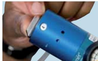
**5.3** Allow the regulator to vent to atmosphere by selecting a flow on the system. **Remove the regulator when the contents gauge reads zero.**
