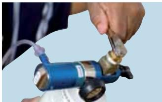
**5.2** Close the cylinder valve using an appropriate cylinder key. **Do not use excessive force.**
