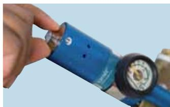
**3.9** Where the regulator or equipment has a flow selector – set the flow selector to the prescribed flowrate.
