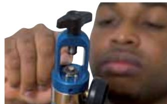
**3.3** Check the Bodok seal is in good condition, clean and free from any signs of oil or grease. **If in doubt, replace with a new one.**
