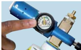
**5.1** Check the cylinder contents gauge to see whether it is empty or has sufficient gas for further use.
