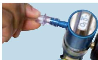
**3.6** Attach appropriate gas delivery equipment if using a regulator. **For example, fit tubing to the fir tree outlet .**
