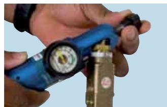
**3.11** With the valve shut, allow residual gas to vent. Remove the yoke and re-inspect the Bodok seal.
