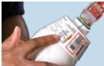
**2.2** Check the expiry date on the batch label fitted to the cylinder.
