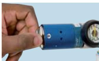
**3.5** Where using a regulator with a flow selector – turn the flow to zero before turning on the gas.
