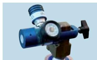
**3.7** Where a regulator is fitted with a Schrader outlet, insert the probe before turning on the cylinder.
