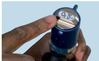
**3.1** Check you have the correct regulator for the medical gas. **Ensure the regulator is not due for any routine maintenance.**
