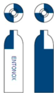
The colour coding of the shoulders of ENTONOX cylinders is quartered blue (RAL 5010) and white (RAL 9010). The colour coding of the cylinder body is white (RAL 9010). Cylinders also carry the ENTONOX name on the body of the cylinder.
