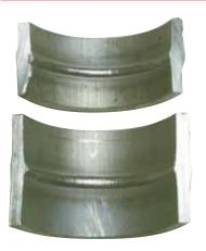
When welding takes place, the temperature of both the parent material and filler rises above the temperature at which oxidation takes place. The shielding gas protects the front of the weld from atmospheric contamination but if no purging or root backing is carried out on the back of the weld, it will oxidise.
