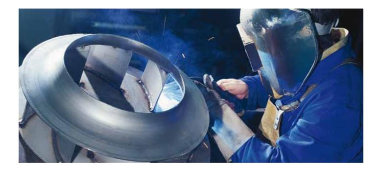
Stainless steel is usually defined as an iron-chromium alloy containing at least 11% chromium. It often contains other elements such as silicon, manganese, nickel, molybdenum, titanium and niobium. Most widely used as corrosion-resistant engineering materials, it finds applications in aggressive environments and at elevated temperatures.
