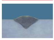
The addition of helium to the shielding gas results in a hotter welding arc than that produced from pure argon.
