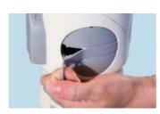
2.4 Remove the tamper evident handwheel cover by pulling the tear ring. Discard the cover into the recycle bin. If the cylinder has been used before this cover will not be present.
